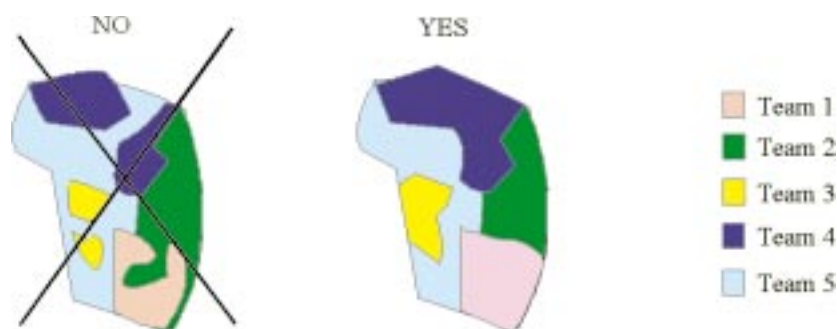
Figure 23 - Splitting the work in zones
